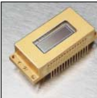
Cooled CCD Sensor— 24 \mu\text{m} sq. pitch, 1100x330 pixel configuration
