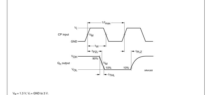
Fig.6 The clock (CP) to output (Q<sub>n</sub>) propagation delays, the clock pulse width, the output transition times and maximum clock pulse frequency.
