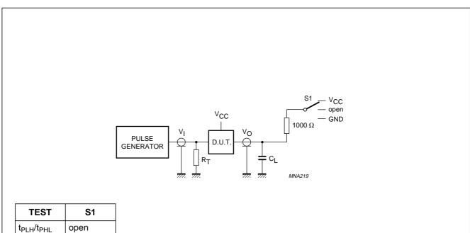
Fig.9 Load circuit for switching times.
