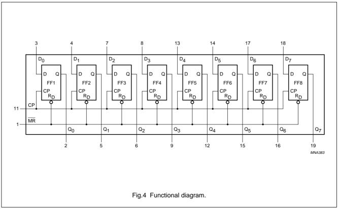
Octal D-type flip-flop with reset; positive edge-trigger; open drain outputs
