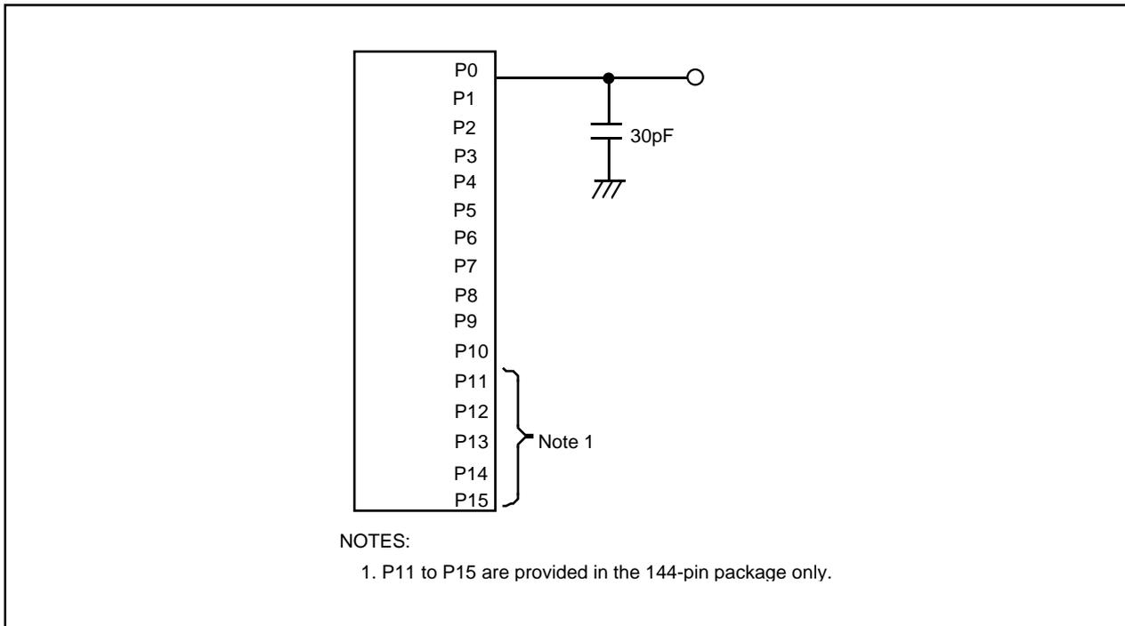
Figure 5.12 P0 to P15 Measurement Circuit
