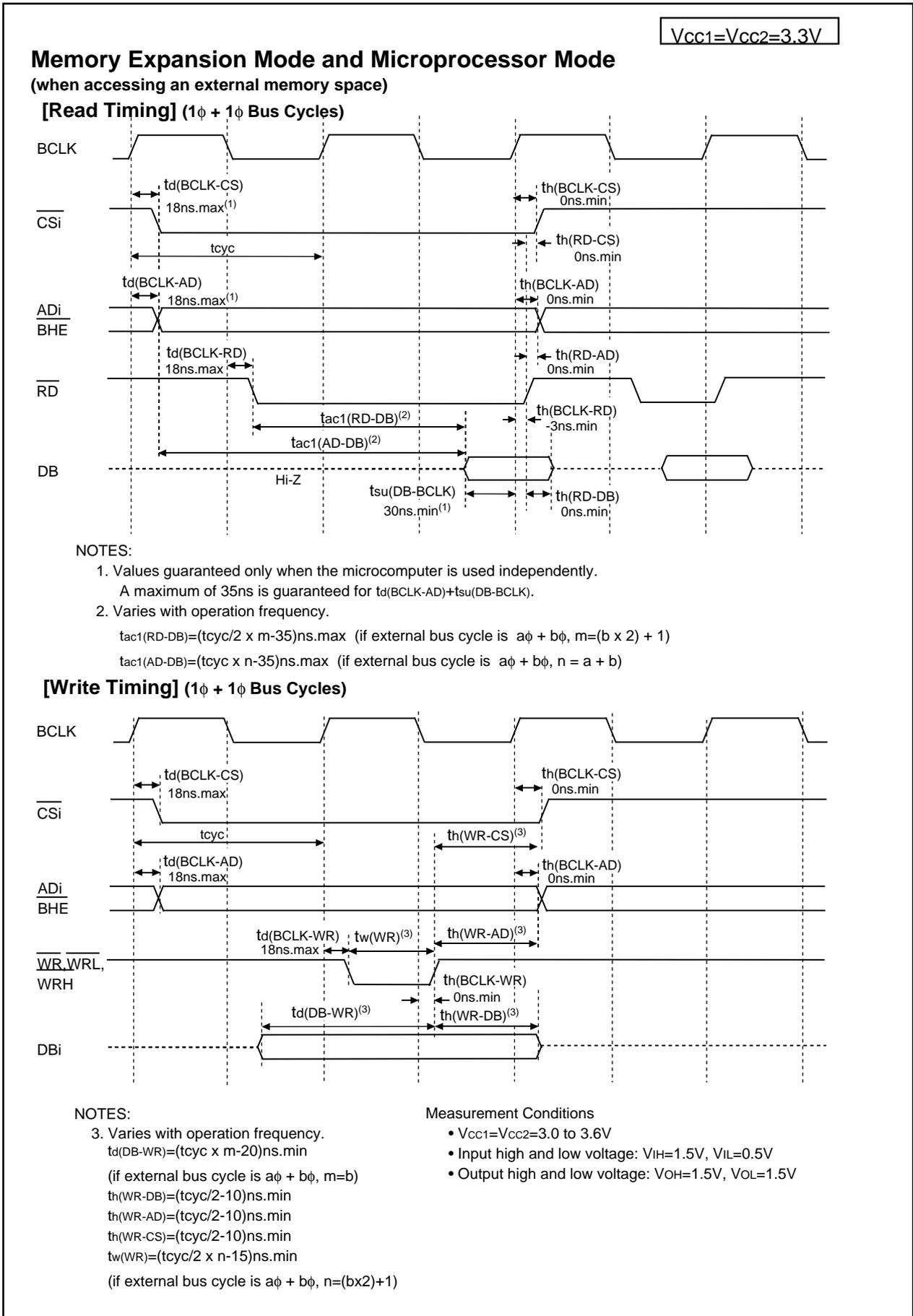
**Figure 5.7 V<sub>CC1</sub>=V<sub>CC2</sub>=3.3V Timing Diagram (1)**
