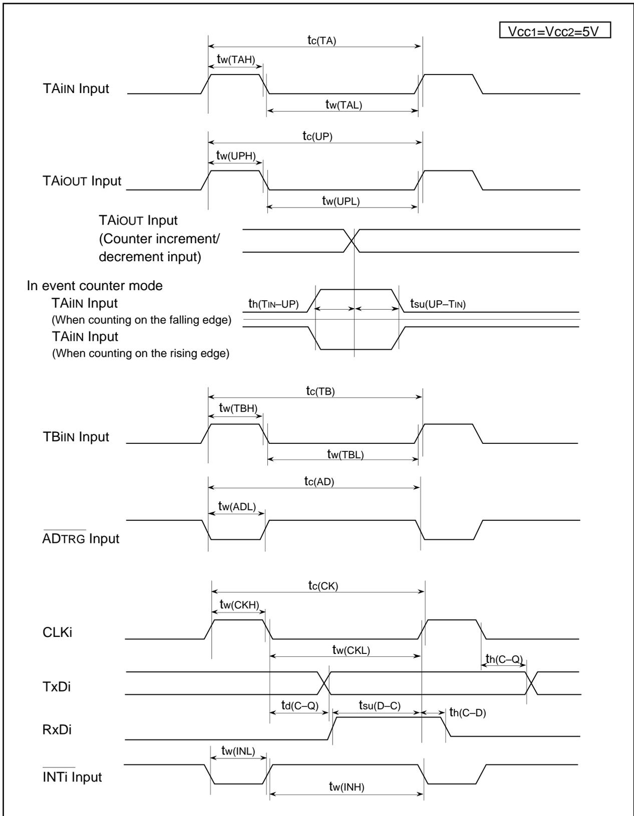
Figure 5.13  $V_{CC1}=V_{CC2}=5V$  Timing Diagram
