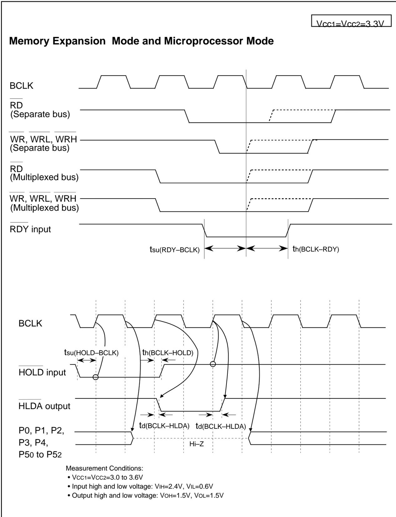
Figure 5.10 V<sub>CC1</sub>=V<sub>CC2</sub>=3.3V Timing Diagram (4)
