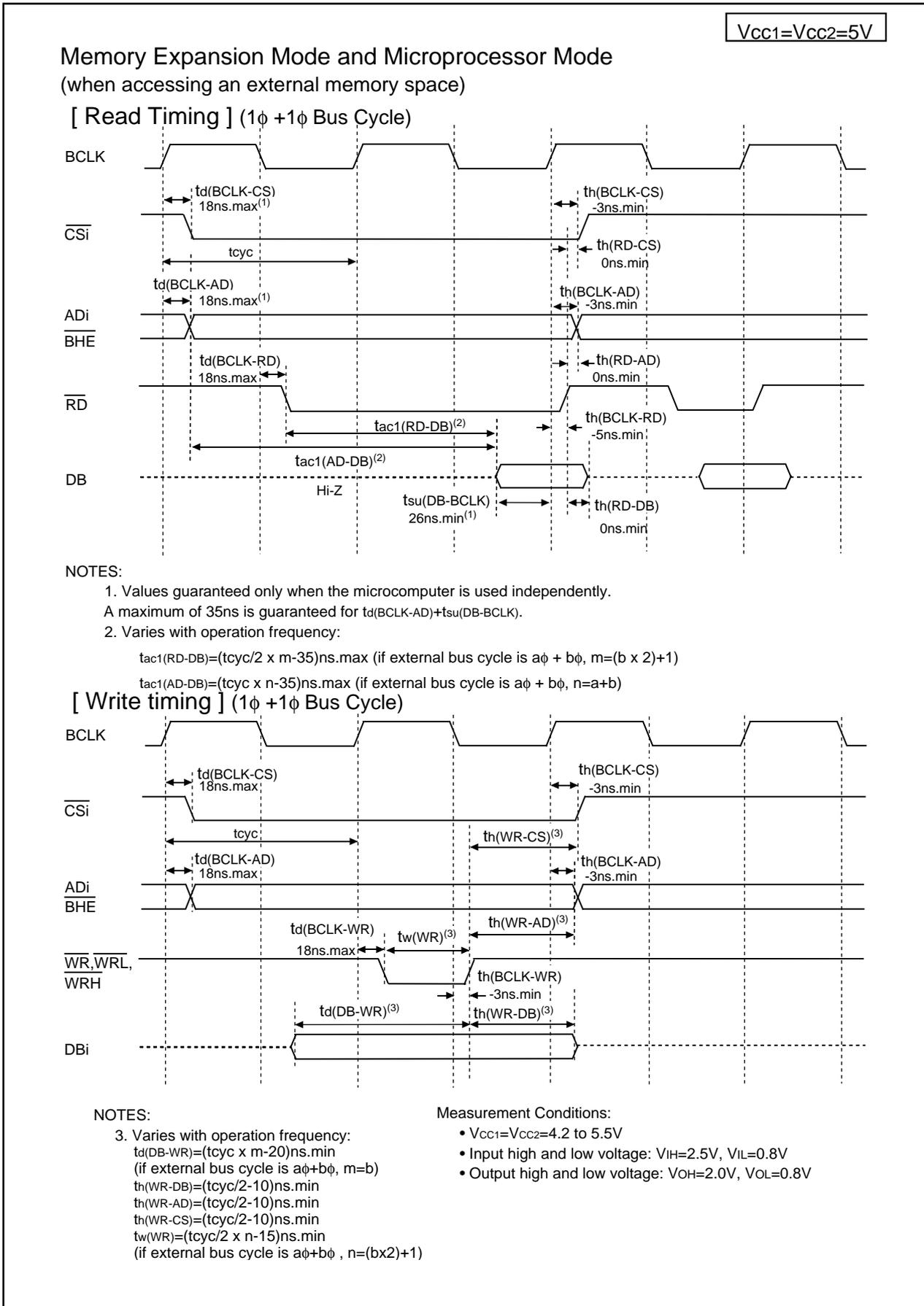
Figure 5.3 V<sub>CC1</sub>=V<sub>CC2</sub>=5V Timing Diagram (1)
