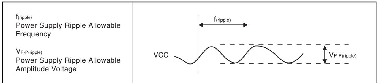
**Figure 5.1 Timing of Voltage Fluctuation**
