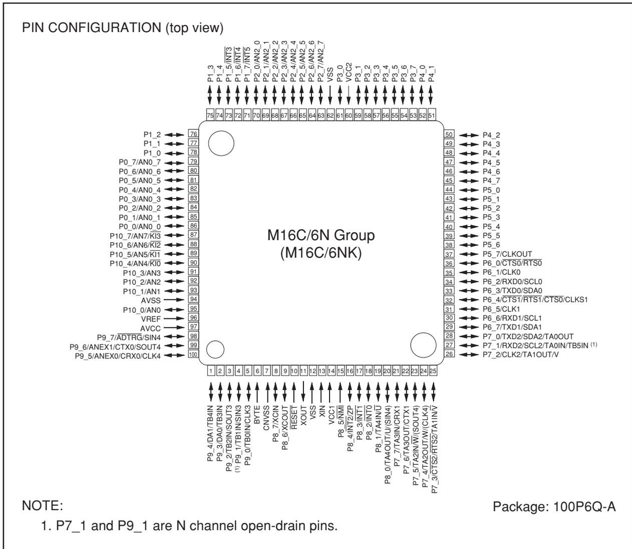
Figure 1.3 Pin Configuration (Top View)
