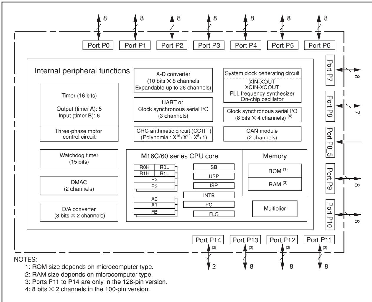
Figure 1.1 Block Diagram
