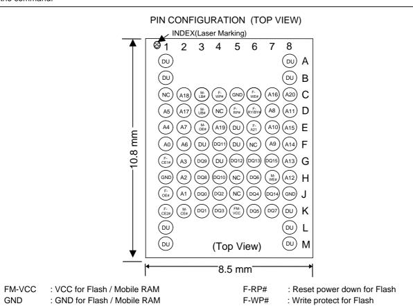
FM-VCC : VCC for Flash / Mobile RAM F-RP# : Reset power down for Flash
