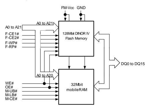
Note: In the 128M-bit DINOR(IV) Flash Memory lower 64Mbit is selected by F-CE1#="L" and upper 64Mbit is done by F-CE2#="L". Never select each chip at the same time. In the data sheet there are "VCC"s which mean "FM-VCC" (Common Vcc for Flash / mobileRAM).
