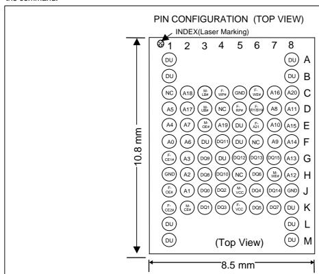
F-VCC : VCC for Flash F-RP# : Reset power down for Flash : VCC for Mobile RAM M-VCC F-WP# : Write protect for Flash : GND for Flash / Mobile RAM **GND** F-RY/BY# : Flash Memory Ready /Busy A0-A20 : Common address for Flash/Mobile RAM M-CE# : Mobile RAM chip enable F-A21 : Address for Flash M-OE# : Output enable for Mobile RAM DQ0-DQ15: Data I/O M-WF# : Write enable for Mobile RAM F-CE1# : Flash chip enable 1 M-LB# : Lower byte control for Mobile RAM F-CE2# : Flash chip enable 2
