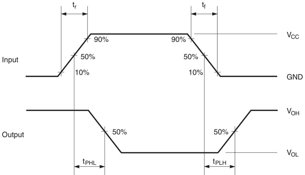
Notes: 1. Input waveform :  $PRR \leq 1$  MHz,  $Z_o = 50 \Omega$ ,  $t_r \leq 3$  ns,  $t_f \leq 3$  ns.
