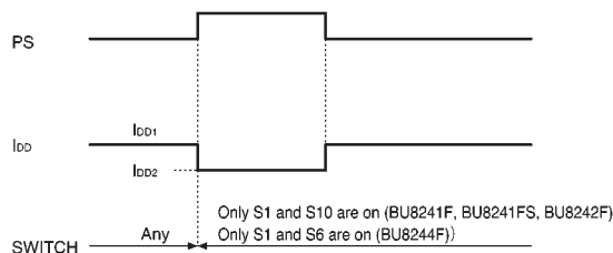
Fig. 3 Power save mode timing waveform
