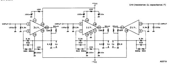
$\begin{array}{ll} \mbox{Vo}: & \mbox{$V_{NO}$ is measured by connecting a VTVM.} \\ & \mbox{$V_{N}$ is measured by connecting a DC voltmeter.} \\ & \mbox{$t_{D}$ is measured by connecting an oscilloscope.} \end{array}$
