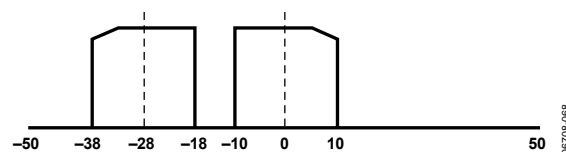
Figure 67. Example AD6653 20 MHz Bandwidth Input Signal Tuned to DC Using the NCO (NCO Frequency = 14 MHz)
