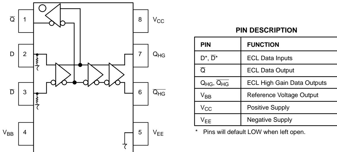
**Figure 1. 8-Lead Pinout (Top View) and Logic Diagram**
