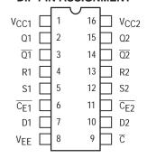
Pin assignment is for Dual–in–Line Package.
