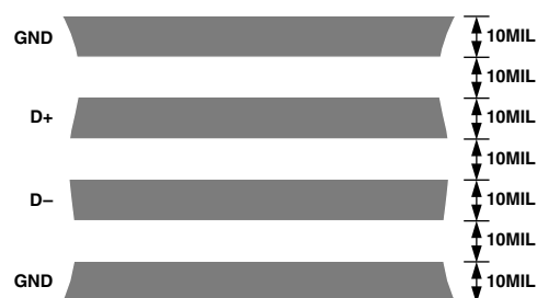
Figure 6. Arrangement of Signal Tracks
