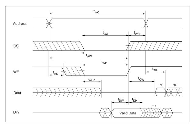
Write Timing Waveform (2) (OE Low Fixed)
