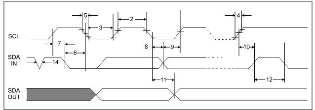
FIGURE 1-2: BUS TIMING START/STOP
