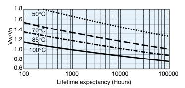
Vw = Working DC Voltage Vn = Rated DC Voltage
