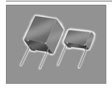
The FFB series uses a non-impregnated metallized polypropylene or polyester dielectric with the controlled self-healing process, specially treated to have a very high dielectric strength in operating conditions up to 100°C.
