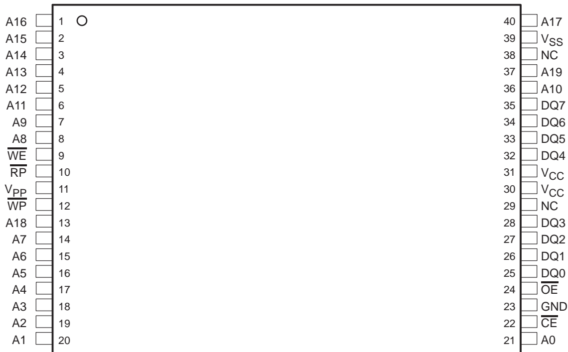
TMS28F008Axy 40-PIN TSOP (DCD) (TOP VIEW)
