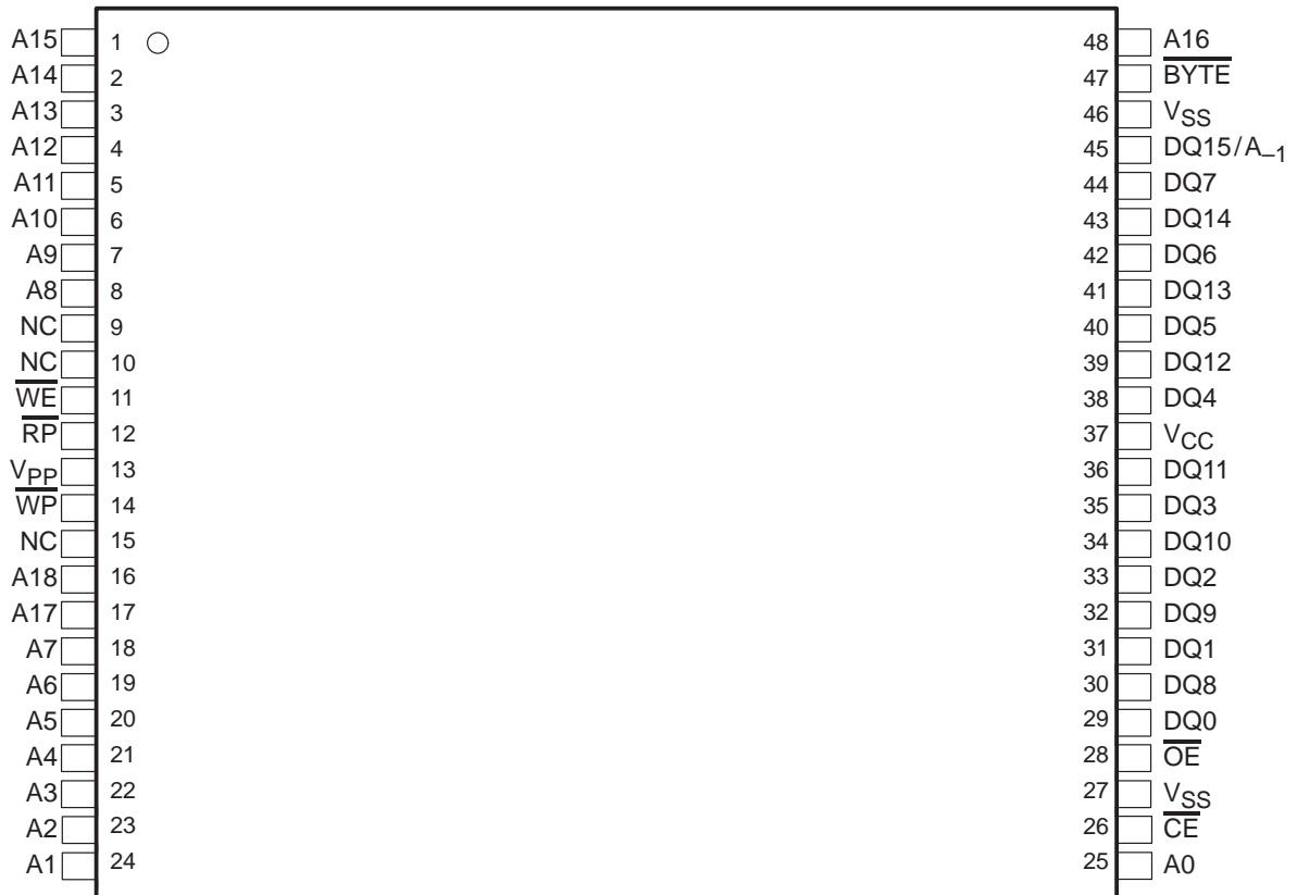
TMS28F800Axy 48-PIN TSOP (DCD) (TOP VIEW)
