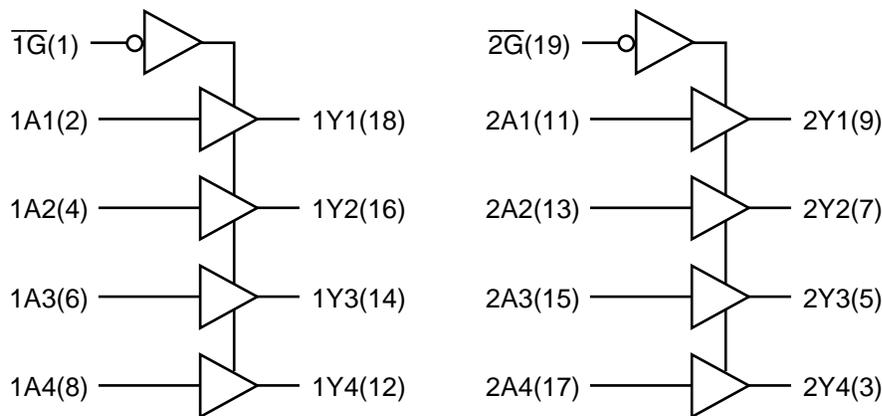
**Figure 2. Pin Configuration**
