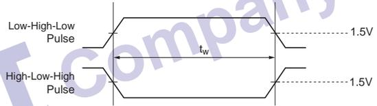
Figure 5. Enable and Disable Timing
