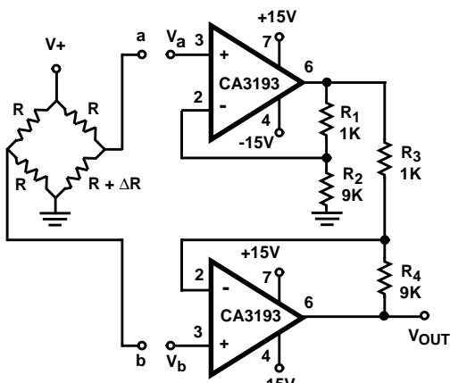
$$V_{OUT} = -V_a \left( \frac{R_2}{R_1 + R_2} \right) + V_b \left( \frac{R_4}{R_3 + R_4} \right)$$
