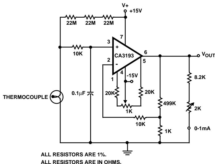
FIGURE 11. THE CA3193 USED IN A THERMOCOUPLE CIRCUIT
