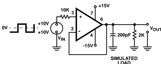
FIGURE 3A. TEST CIRCUIT
