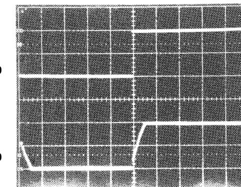
Top Trace: Input Voltage; Bottom Trace: Output Voltage
