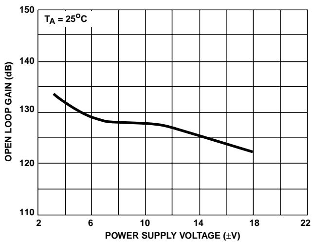
FIGURE 19. OPEN LOOP GAIN vs POWER SUPPLY VOLTAGE
