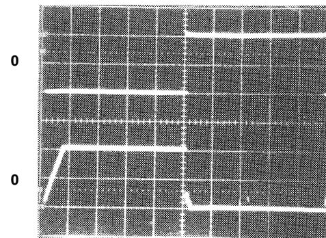
Top Trace: Input Voltage; Bottom Trace: Output Voltage
