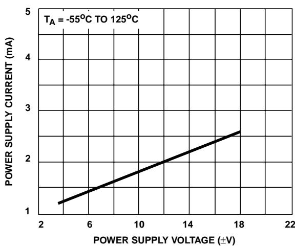
FIGURE 17. POWER SUPPLY CURRENT vs SUPPLY VOLTAGE
