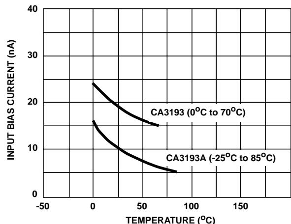
FIGURE 14. TYPICAL INPUT BIAS CURRENT vs TEMPERATURE
