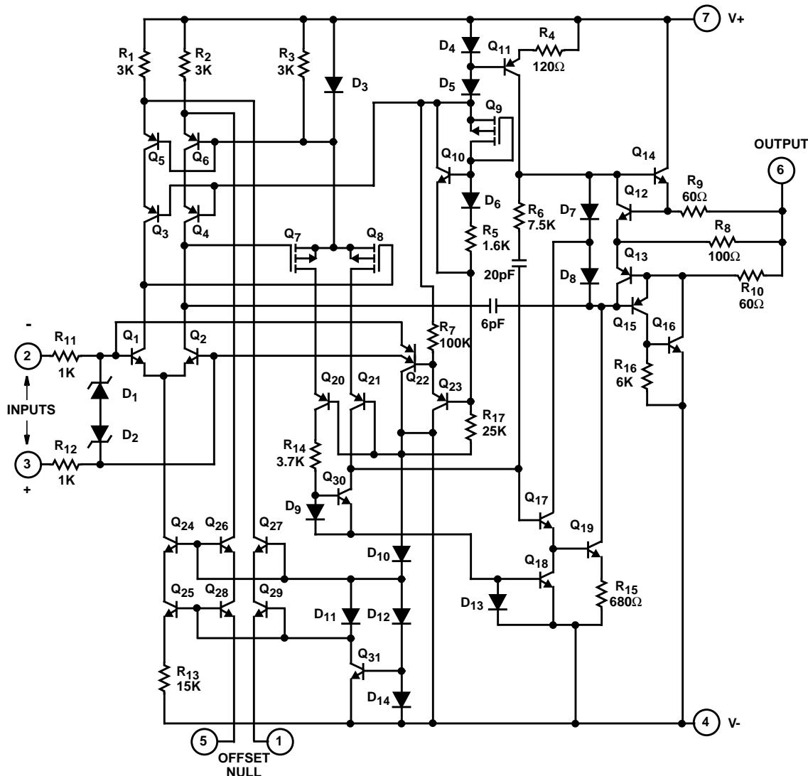
FIGURE 6. SCHEMATIC DIAGRAM OF CA3193A AND CA3193
