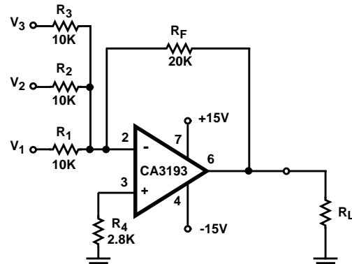
$$V_{OUT} = - \left( \frac{R_F}{R_1} V_1 + \frac{R_F}{R_2} V_2 + \frac{R_F}{R_3} V_3 \right)$$
