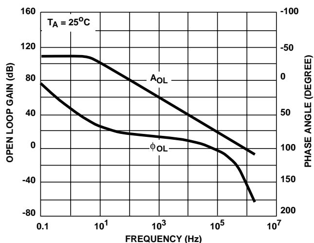
FIGURE 18. OPEN LOOP GAIN AND PHASE SHIFT RESPONSE
