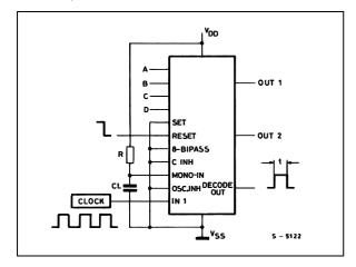
Time Internal Configuration Using On-Chip RC oscillator and Reset Input to Initiate Time Interval
