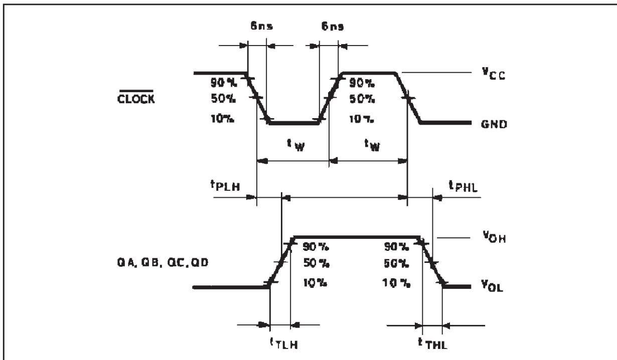
WAVEFORM 2 : MINIMUM SETUP AND HOLD TIME (f=1MHz; 50% duty cycle)
