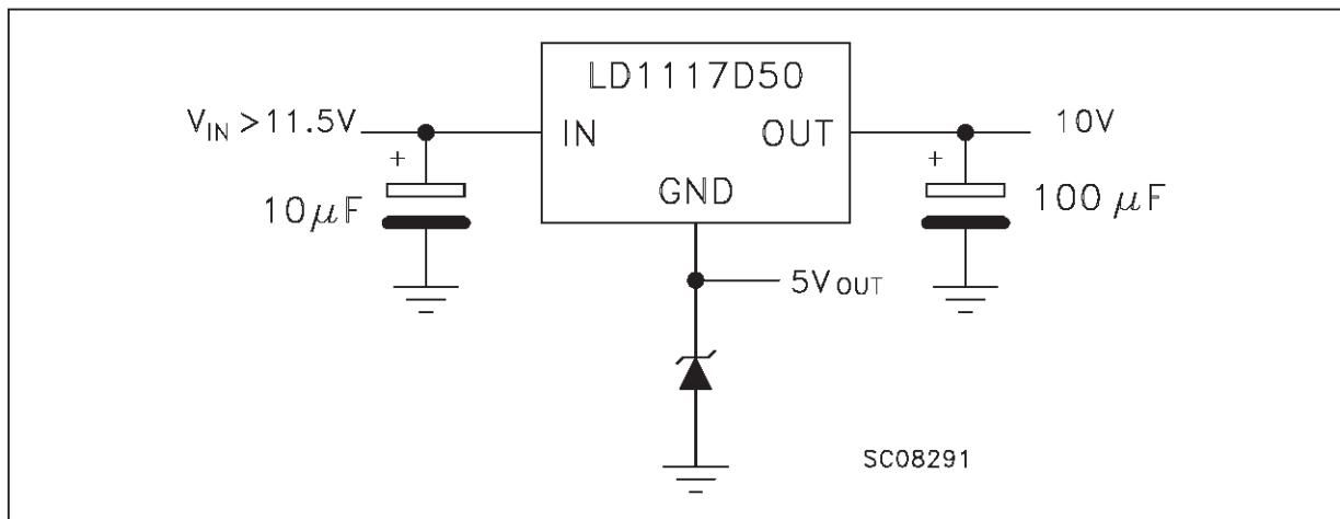
**FIGURE 5:** Battery Backed-up Regulated Supply
