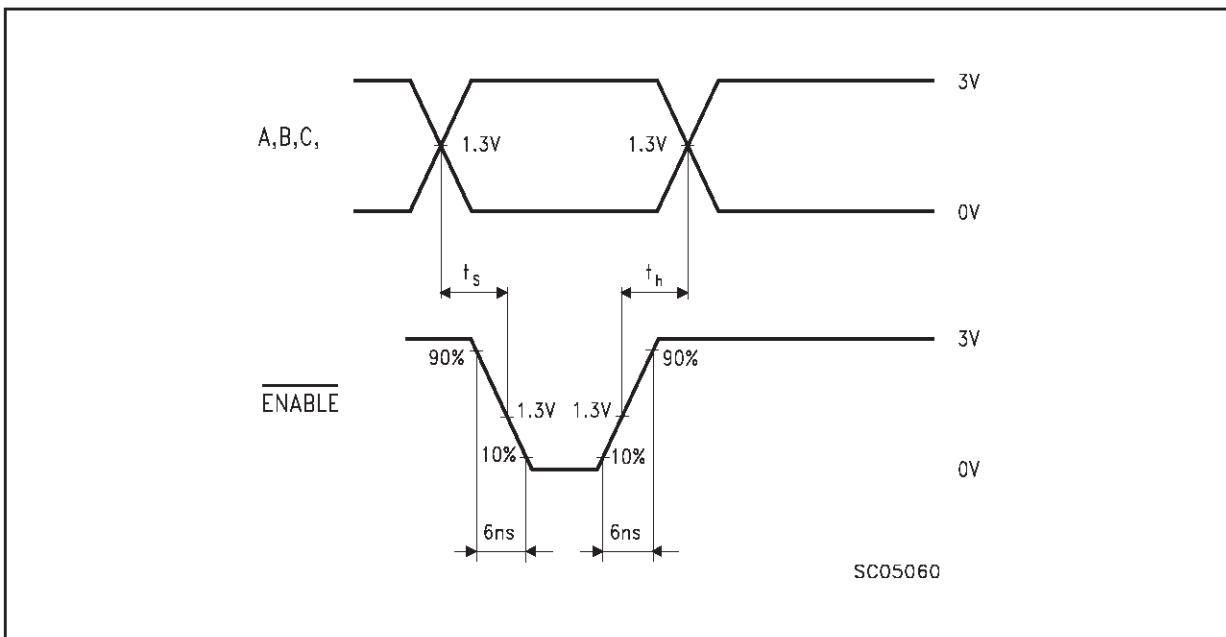
**INPUT WAVEFORMS (f=1MHz; 50% duty cycle)**
