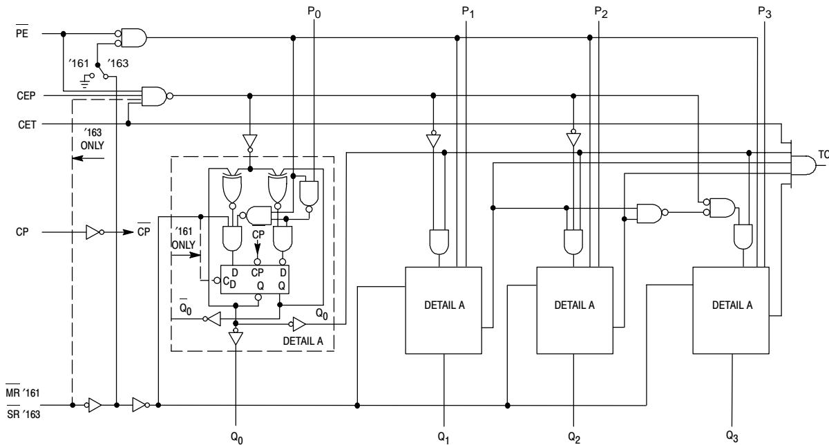
NOTE: This diagram is provided only for the understanding of logic operations and should not be used to estimate propagation delays.
