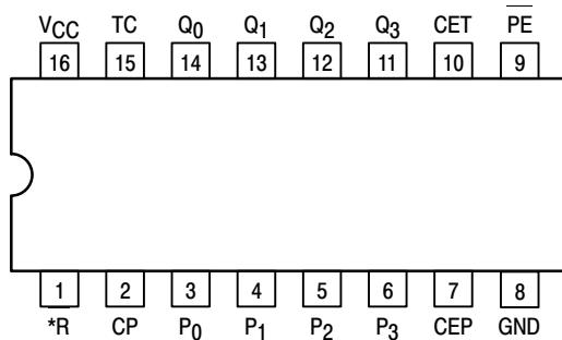
Figure 1. Pinout: 16-Lead Packages Conductors
