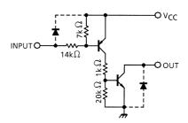
Note: The input and output parasitic diodes cannot be used as clamp diodes.
