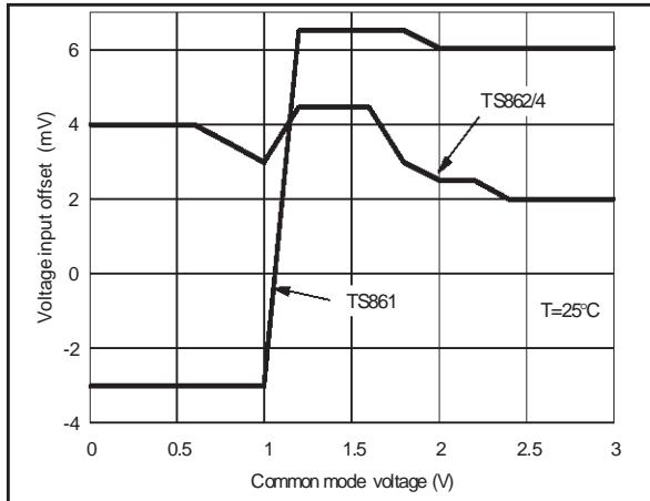
$V_{IO}$  versus  $V_{ICM}$  and temperature at  $V_{CC} = 2.7V$
