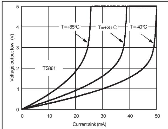
**V<sub>OH</sub> vs I<sub>SOURCE</sub> and temperature at V<sub>CC</sub>=5V**
