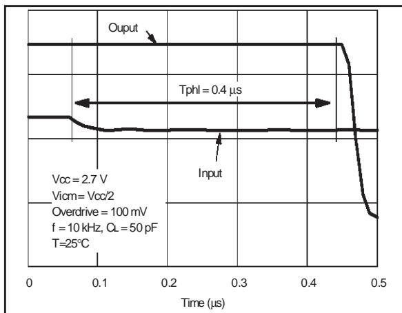
**Response time T<sub>PLH</sub> at V<sub>CC</sub>= 2.7V**
