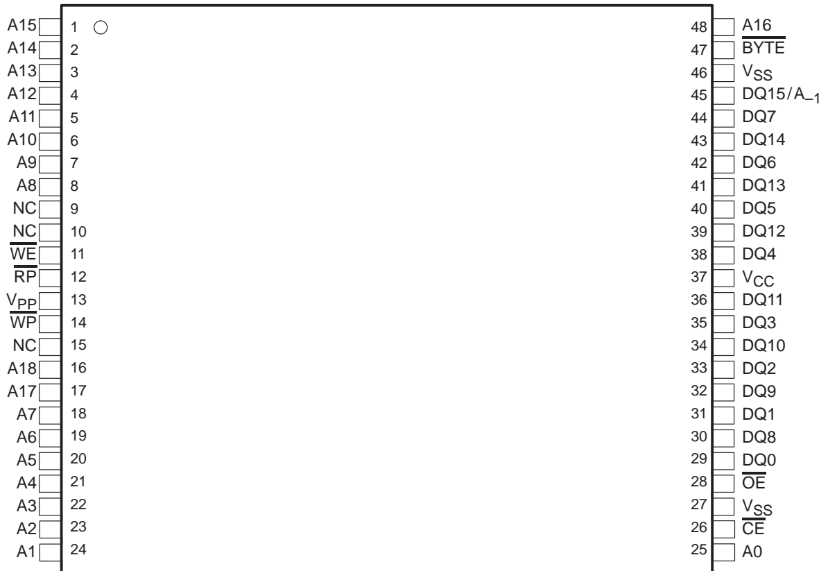
TMS28F800Axy 48-PIN TSOP (DCD) (TOP VIEW)
