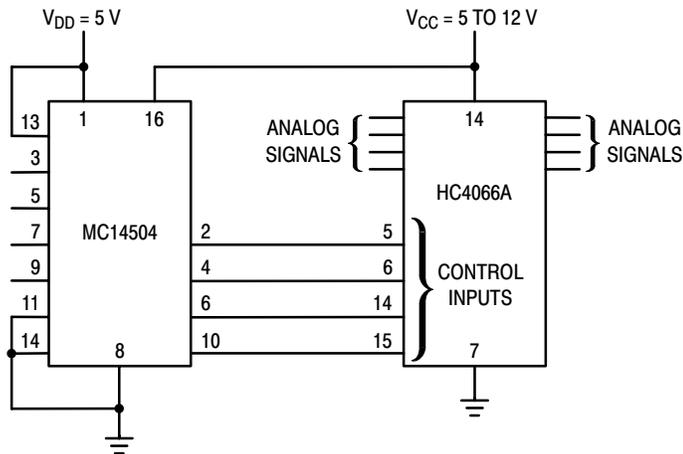
Figure 19. TTL/NMOS-to-CMOS Level Converter
