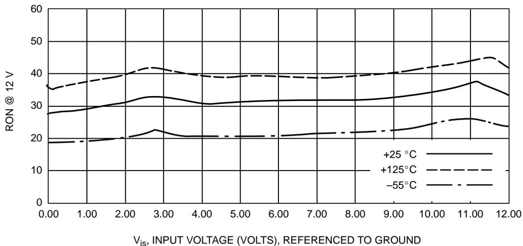
**Figure 1f. Typical On Resistance,  $V_{CC} = 12.0$  V**
