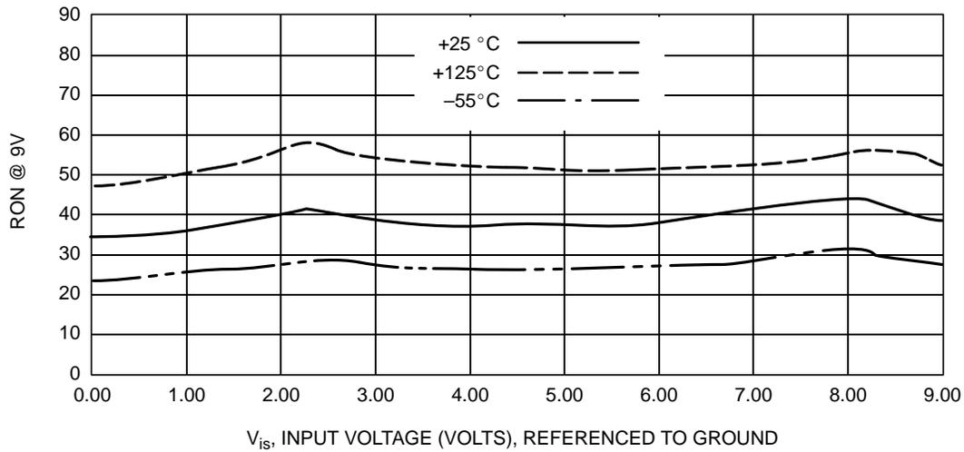
**Figure 1e. Typical On Resistance,  $V_{CC} = 9.0$  V**
