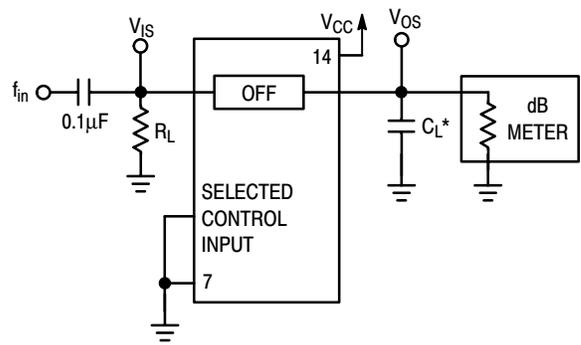
\*Includes all probe and jig capacitance.
