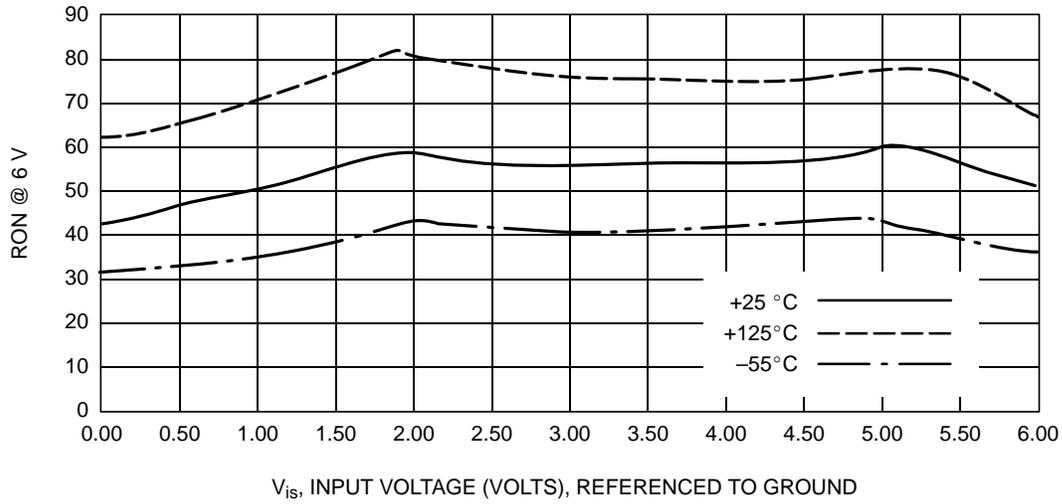
**Figure 1d. Typical On Resistance,  $V_{CC} = 6.0$  V**
