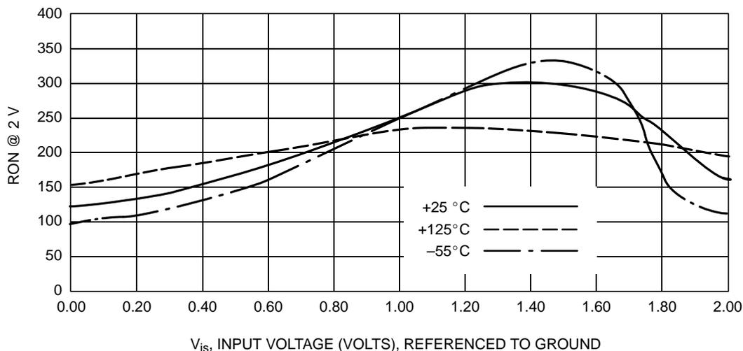
**Figure 1a. Typical On Resistance, V<sub>CC</sub> = 2.0 V**
