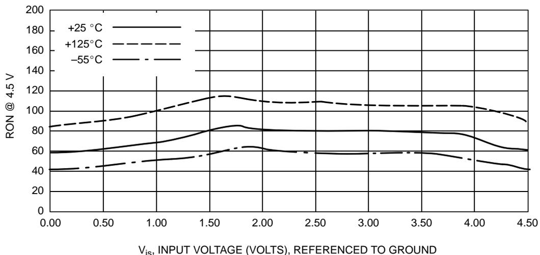
**Figure 1c. Typical On Resistance, V<sub>CC</sub> = 4.5 V**
