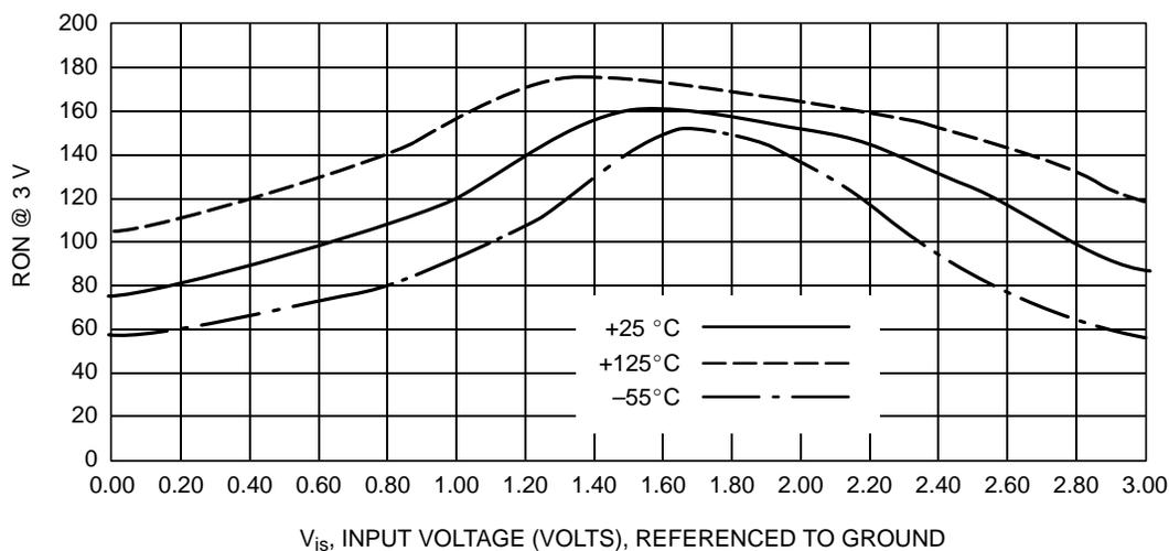
**Figure 1b. Typical On Resistance, V<sub>CC</sub> = 3.0 V**
