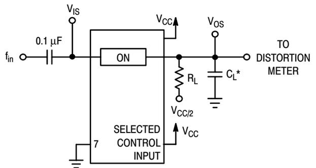
\*Includes all probe and jig capacitance.
