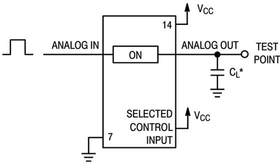
\*Includes all probe and jig capacitance.
