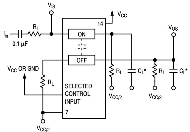
\*Includes all probe and jig capacitance.
