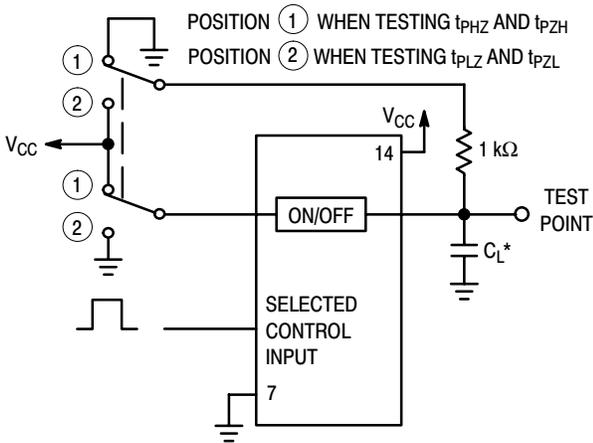
\*Includes all probe and jig capacitance.
