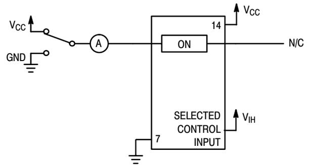
Figure 4. Maximum On Channel Leakage Current, Test Set-Up
