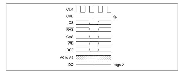
Self refresh command (REF): If both banks are in idle state, at the CLK rising edge, by setting CS, RAS, CAS, DSF; LOW, WE; HIGH, and if CKE's falling edge is detected, the HM5283206 starts self-refresh operation. Self-refresh operation is kept while CKE is LOW. [State transition] Idle — (Self refresh command) -> Self refresh mode
