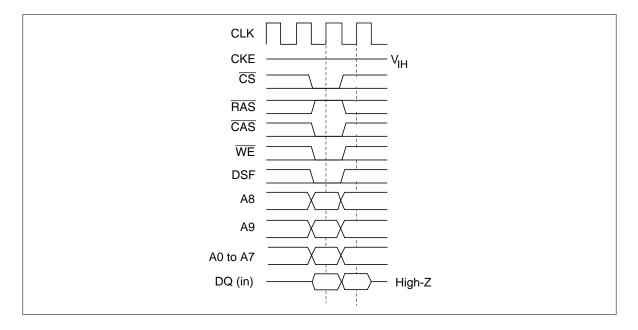
**Burst stop command (BST):** At the CLK rising edge, by setting  $\overline{CS}$ ,  $\overline{WE}$ , DSF: LOW,  $\overline{RAS}$ ,  $\overline{CAS}$ ; HIGH, full page burst (BL = 256) read/write is interrupted. If BL is set to 1, 2, 4, 8, to try to execute this command is illegal. [State transition] Row active — (Burst stop command) -> Row active
