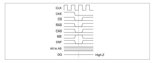
No operation command (NOP): At the CLK rising edge, by setting  $\overline{CS}$ ; LOW, WE, RAS,  $\overline{CAS}$ ; HIGH, [State transition] No transition
