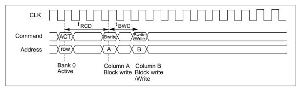
2. Operation for a column in other row of the same bank: It is necessary to execute a precharge command and a bank active command before the following write or another block write operation.
