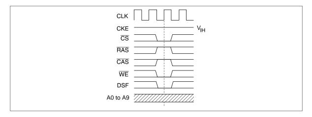
Auto refresh command (REF): If both banks are in idle state, at the CLK rising edge, by setting  $\overline{CS}$ ,  $\overline{RAS}$ ,  $\overline{CAS}$ , DSF; LOW,
