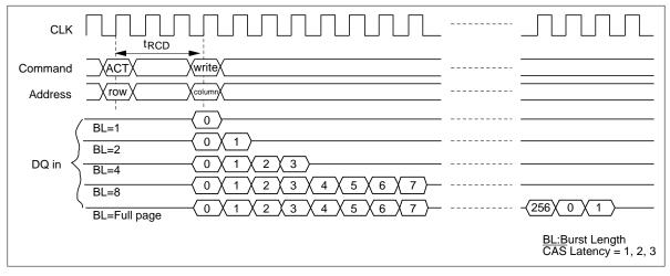
**Single write:** Before executing a single write operation, OPCODE (A9, A8) should be set to (1, 0). In the single write operation, data are only written to the single column defined by the column address and the bank select address loaded at the write command set cycle regardless of the defined burst length. (The latency of data input is 0).
