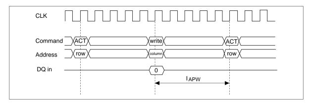
**Block write with auto-precharge:** In this operation, since precharge is automatically performed after completion of a block write operation, so no need to execute precharge command. The following command must be a bank active command (ACTV, ACTVM). In addition, an interval of  $l_{APBW}$  is required between the last valid data input and the following command.
