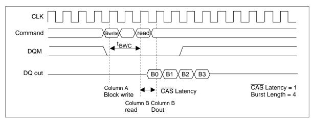
2. Operation for a column in other row of the same bank: It is necessary to execute a precharge command and a bank active command before the following write or another block write operation.
