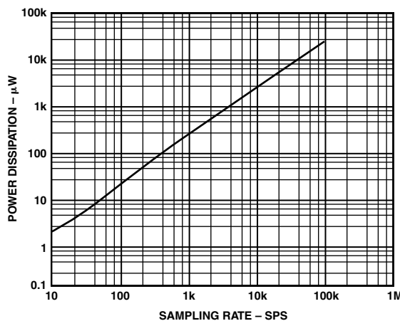
Figure 10. Power Dissipation vs. Sample Rate
