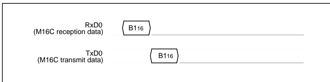
Figure 1.25.30. Timing of baud rate 19200
