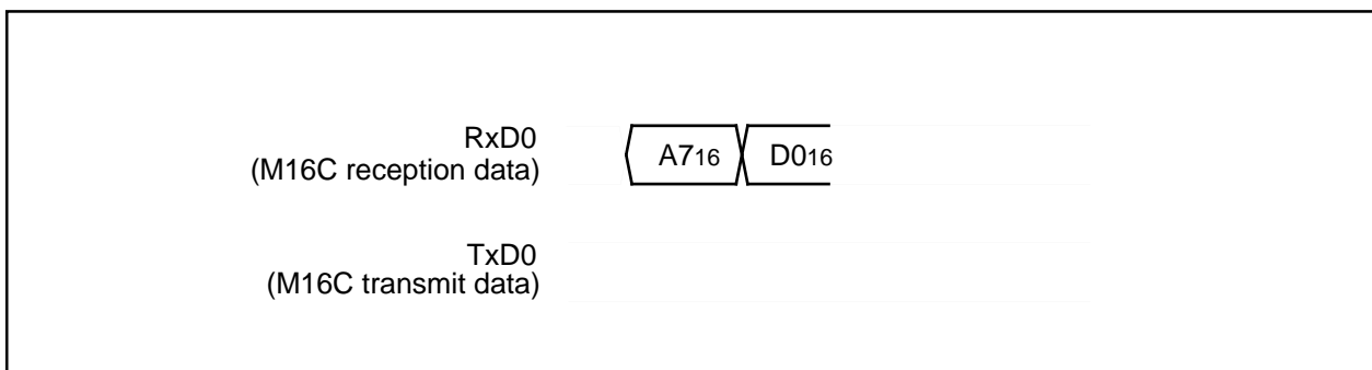
Figure 1.25.22. Timing for erasing all blocks
