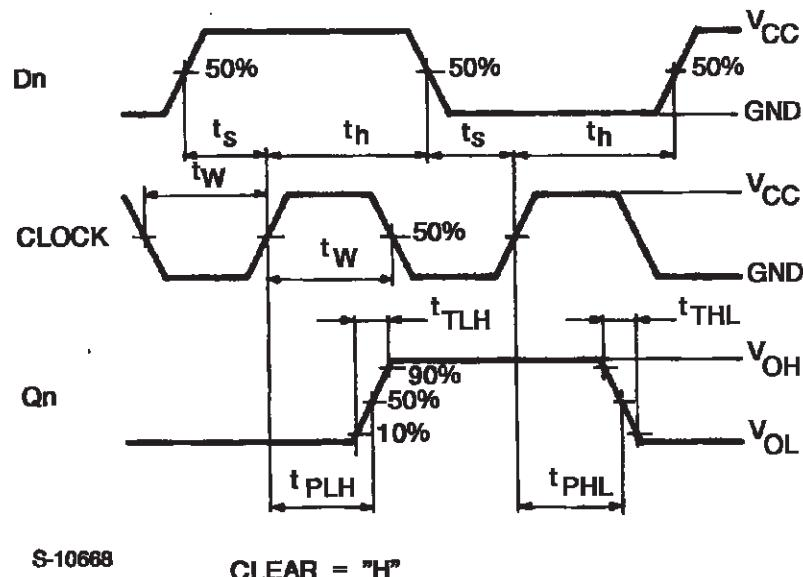
**WAVEFORM 2: MINIMUM PULSE WIDTH (CLEAR) AND REMOVAL TIME (CLEAR TO CLOCK) (f=1MHz; 50% duty cycle)**
