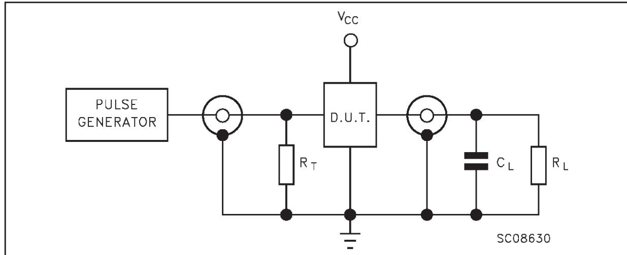
$C_L = 50$  pF or equivalent (includes jig and probe capacitance)
