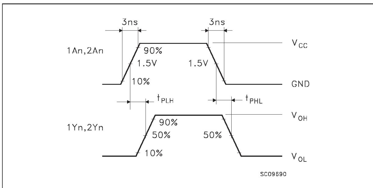
**WAVEFORM 2: OUTPUT ENABLE AND DISABLE TIME (f=1MHz; 50% duty cycle)**
