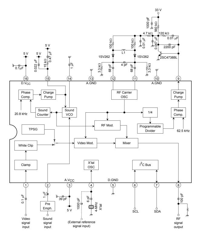
L1: Coil diameter = 3.2 mm, wire diameter = 0.4 mm, 2.5 turns
