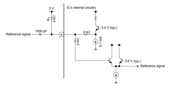
In this case, configure  $R_1$  and the external circuitry so as to ensure that a voltage of at least 3.8 V is applied to pin 4 and that the sine-wave reference signal has an amplitude of at least 100 mVp-p.
