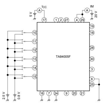
I<sub>CC</sub>1, IM1: Upper phase 1 ON, lower phase 1 ON (eg, U-phase: H; V-phase: L; W-phase: Z) I<sub>CC</sub>2, IM2: Upper phase 1 ON, synchronous regeneration mode (eg, U-phase: H; V-phase: H; W-phase: Z) I<sub>CC</sub>3, IM3: All phases OFF
