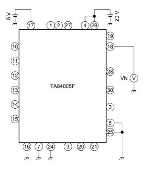
Test Circuit 9: VCMP, VOL (CMP), ROH (CMP)
