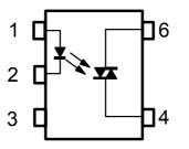
1: ANODE 2: CATHODE 3: N.C. 4:TERMINAL1 6:TERMINAL2
