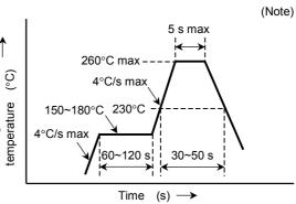
• Please perform the first reflow soldering with reference to the above temperature profile and within 168 h of opening the package.
