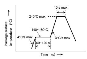
Recommended Temperature profile for Pb-free soldering
