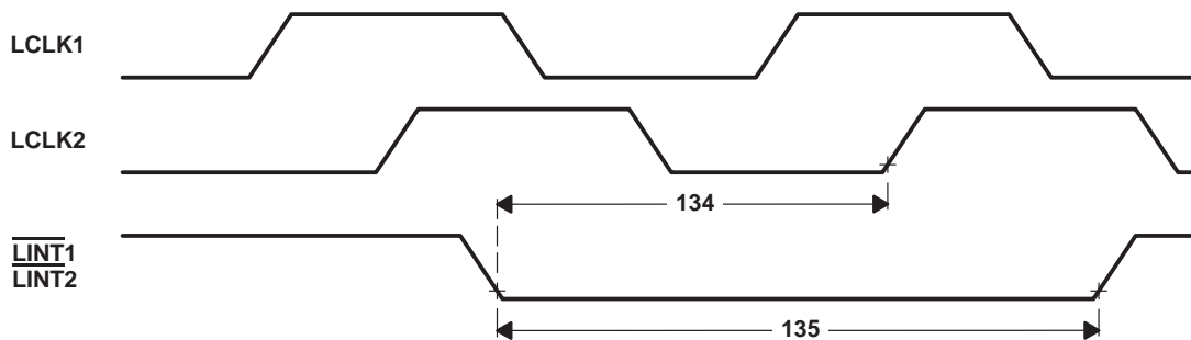
Figure 56. Interrupt Timing: \overline{LINT1} and \overline{LINT2}
