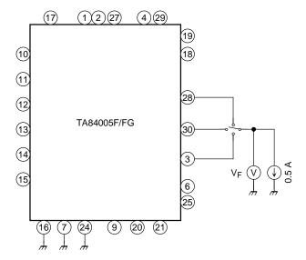
Test Circuit 7: V<sub>F</sub> (H)
