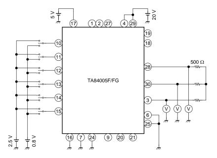
Input  $V_{\mbox{IN}}$  = 0.8 V/2.5 V, measure the output voltage, and test the function.
