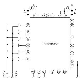
ICC1, IM1: upper phase 1 ON, lower phase 1 ON (e.g., U-phase: H; V-phase: L; W-phase: Z)
