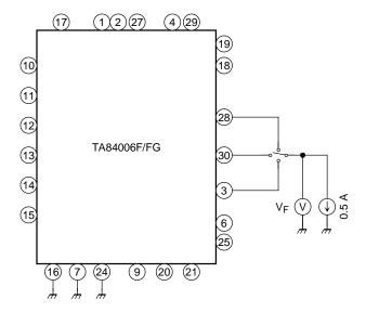
Test Circuit 7: V<sub>F</sub> (H)
