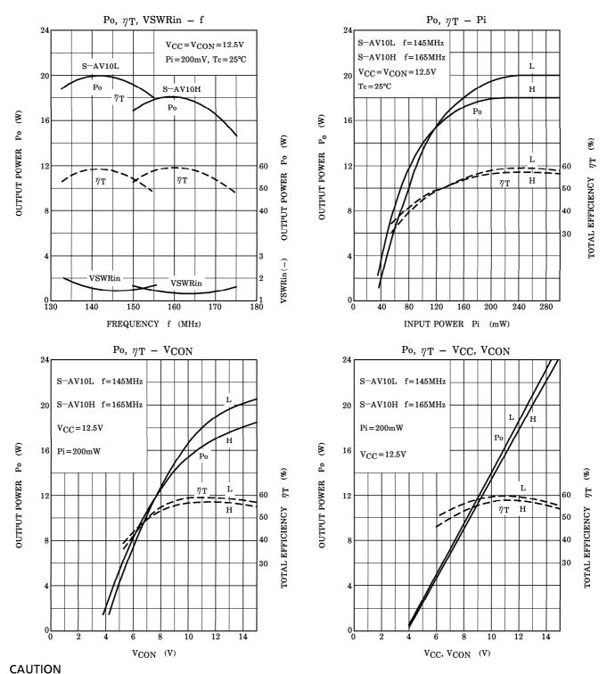
These are only typical curves and devices are not necessarily guaranteed at these curves.
