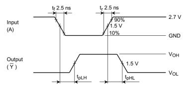
Figure 2 t<sub>pLH</sub>, t<sub>pHL</sub>
