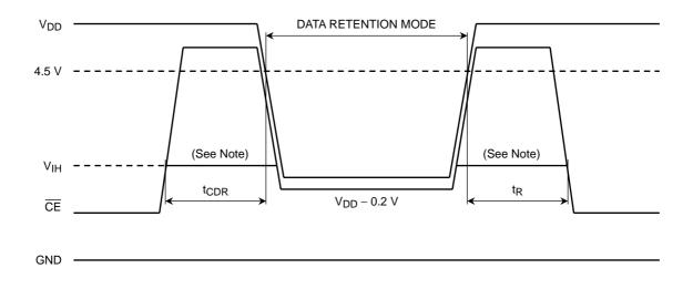
Note: When  $\overline{CE}$  is operating at the VIH level (2.2V), the standby current is given by IDDS1 during the transition of VDD from 4.5 to 2.4V.
