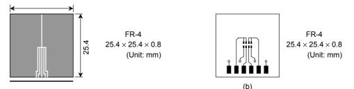
(b) Device mounted on a glass-epoxy board (b)
