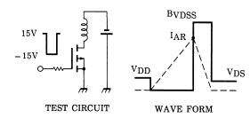
$$\begin{array}{ll} R_G\!=\!25\Omega \\ V_{DD}\!=\!-25V,\; L\!=\!10mH \end{array} \qquad E_{AS}\!=\!\frac{1}{2}\cdot L\cdot I^2\cdot (\frac{B_{VDSS}}{B_{VDSS}\!-V_{DD}}) \end{array} \label{eq:RG}$$
