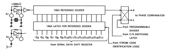
The programmable divider is composed of binary 14 bits and is capable frequency division from 5 to ٠ 16,383 divisions by serial data given externally.
