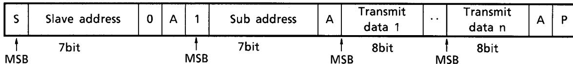
In this transmission method, data is set on automatically incremented sub-address from the specified sub-address.
