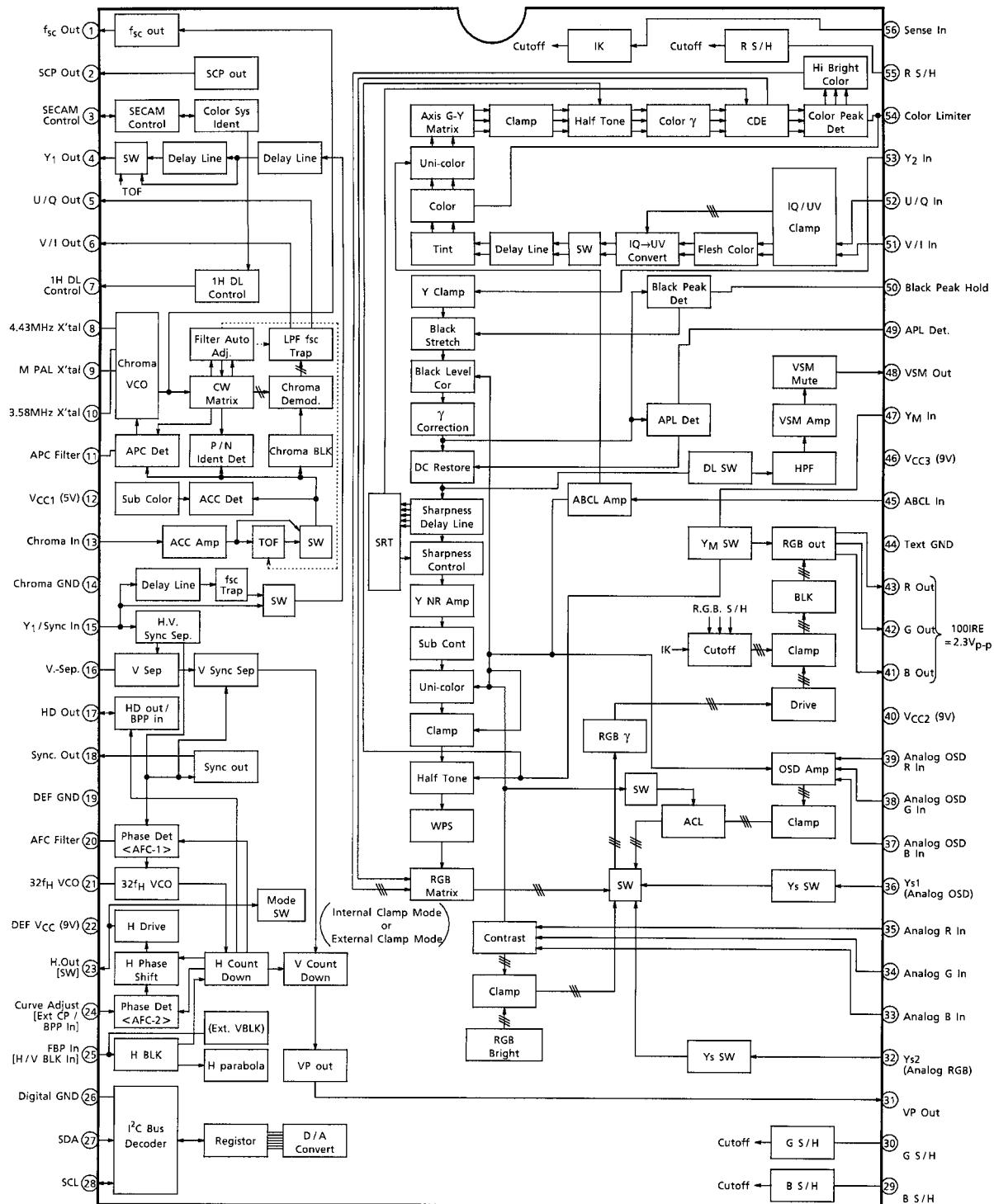
● Pin 23 connect to V<sub>CC</sub> : Double Scan mode
