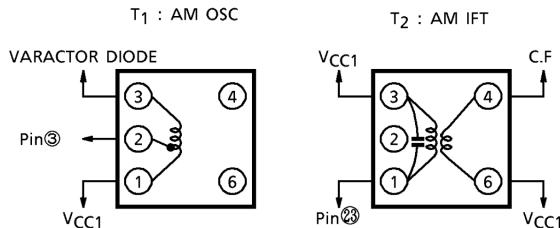
**Test Circuit 2**
